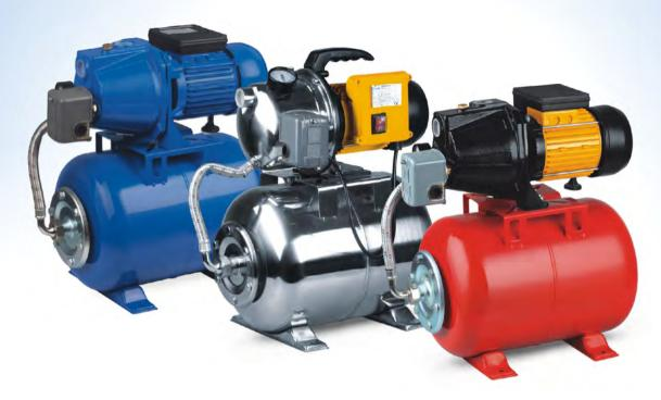
The automatic booster systems consist of a JET water pump, a pressure tank, an airtight pressure switch, a pressure gauge and a connecting flexible pipe. make the pump automatic more convenient to use. The pressure tank, equipped with a non-toxic rubber membrane, has been pre-filled with air pressure of approx 0.12 MPa before leaving the factory.
